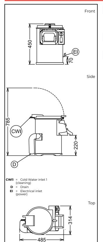
Electric Supply voltage: 603501 (DT5S) 220-240 V/1N ph/50/60 Hz Electrical power max.: 0.12 kW **Total Watts:** 0.12 kW Capacity: Performance (up to): 80 kg/hour 5 litres Capacity: Key Information: External dimensions, 314 mm Width: External dimensions, Depth: 485 mm External dimensions, Height: 450 mm
